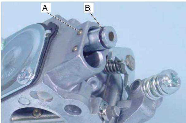
7. Temporarily insert new limiter caps on both L and H mixture needle by aligning groove on limiter cap (B) to locating pin (A) on extension housing. Make it sure that limiter cap face is leveled with extension housing top. Do not press limiter cap deeper at this moment.
