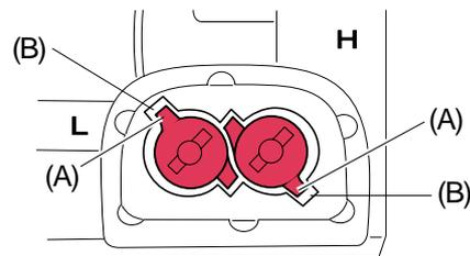
2. Screw 2.5 mm wood screw in the center of the L limiter cap.
