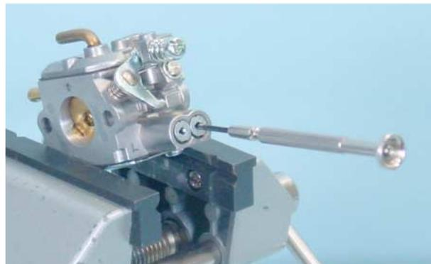
8. Turn L and H mixture needles clockwise until lightly seated using 1.5mm blade screw driver, and then turn both needles anticlockwise for following turns.
