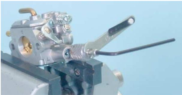
5. While holding bolt with L wrench, turn the nut clockwise to take out the limiter cap.
