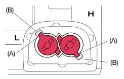
**NOTE**: Align the limiter cap's tabs (A) with locating slots (B) in extended housing of carburettor.
