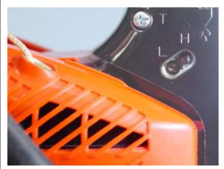
5. Turn L and H mixture needle clockwise until lightly seated, and then turn both mixture needles anticlockwise following turns.
