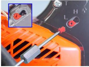
4. Screw thread of limiter cap tool 91019 into other centre hole of the other limiter cap anticlockwise until the limiter cap is come out from the mixture needle completely. Remove the limiter cap from limiter cap tool turning clockwise. Screw thread of limiter cap tool 91019 into centre hole of previous limiter cap to pull out completely.
