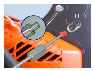
8. After adjusting carburettor, put new limiter cap on the other side of limiter cap tool as shown, and press the limiter caps to the bottoms on L and H mixture needles respectively.
