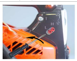
1. Turn the L and H mixture needles anticlockwise to rich side stop and meet limiter caps tabs (A) with locating slot (B), using 3 mm blade screw driver.
