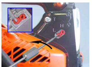
2. Screw left hand thread of limiter cap tool 91019 into centre hole of limiter cap anticlockwise until tab of the limiter cap just come out from locating slot.
