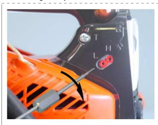
3. Remove the limiter cap tool from the limiter cap turning the tool clockwise as the limiter cap is remained there.
