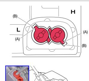
1. Remove cleaner lid. Turn the L and H mixture needles anticlockwise to rich side stop and meet limiter caps tabs (A) with locating slot (B), using 3 mm blade screw driver.
