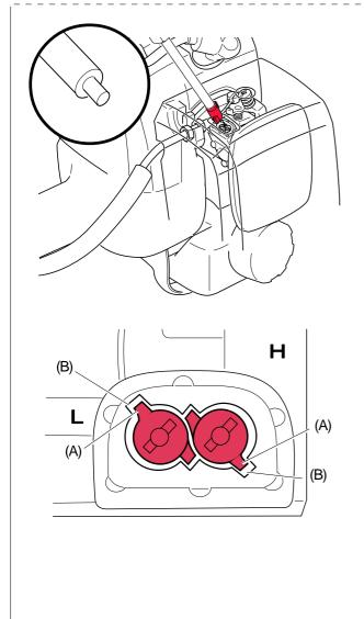
8. After adjusting carburettor, put new limiter cap on the other side of limiter cap tool as shown, and press the limiter caps to the bottoms on L and H mixture needles respectively.
