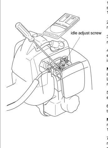
1. Start engine and warm it up alternating engine speed between WOT and idle every 5 seconds for 1 minute.
