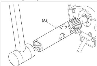
NOTE: Do not reuse removed worm gear. Bore of the used worm gear may be enlarged and the worm gear may slip on sprocket shaft.
